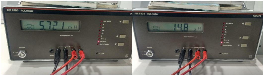
Fig. 38. Measurements of the inductances of the transformer.
