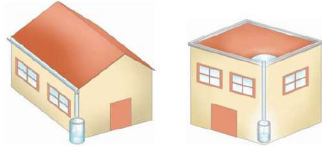
Illustration 5 Examples of collecting rain water out of the roofs. Source: Secretaría de Medio Ambiente de México.
