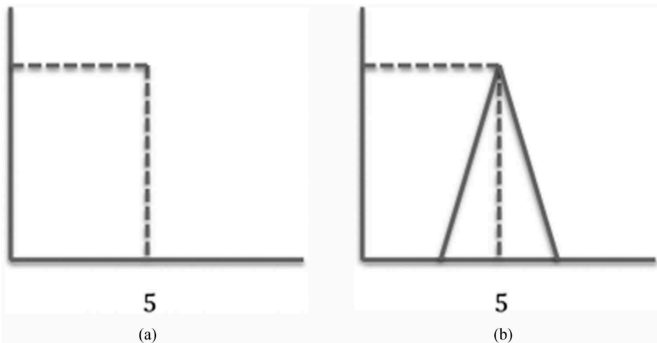
Figure 1. Representation of (a) crisp time 'five o'clock', (b) fuzzy time 'about five'.
