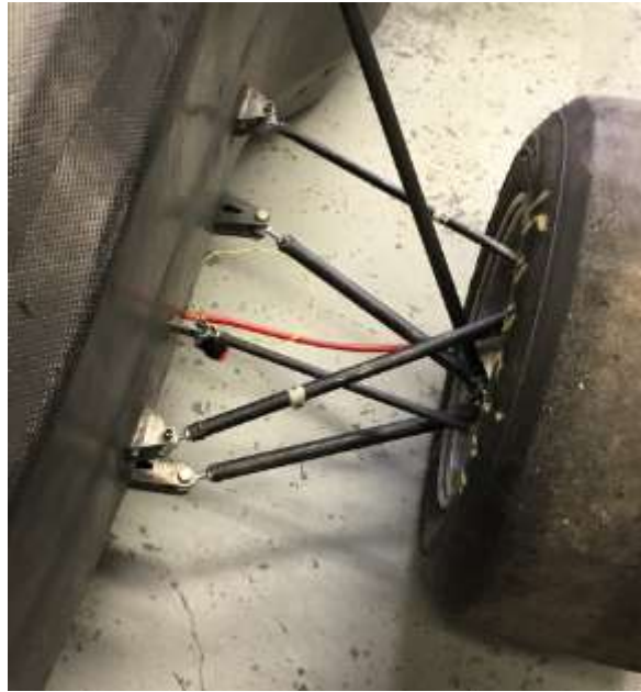
Figure 9.3.5: Front left corner of TR19's car showing the adjustable control arms
