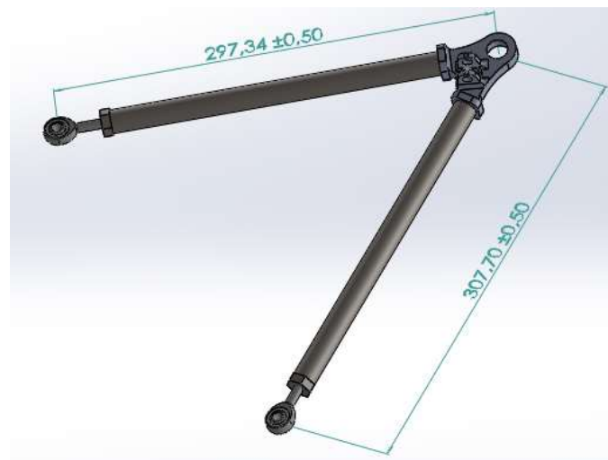
Figure 7.3.3: Front Lower Control Arm assembly (XDRI)
