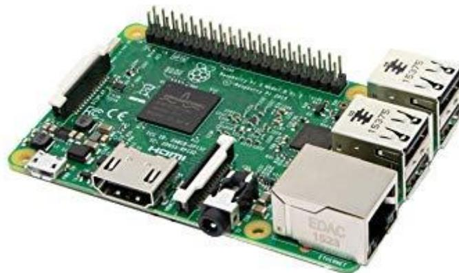
Figura 26: Microcontrolador Raspberry Pi 3B [17]
