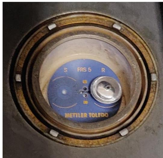
Figure 11: Differential scanning calorimetry probe arranged in the DSC822
