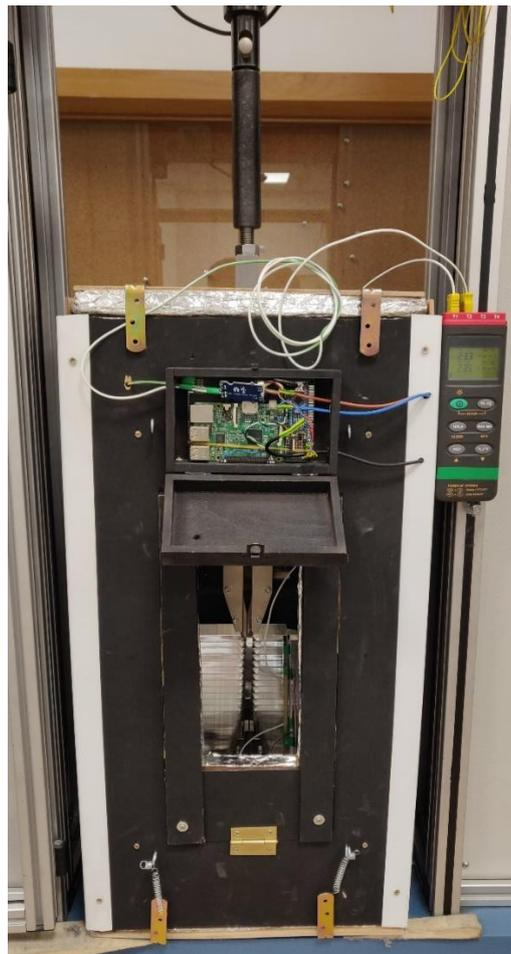
*Figure 7: Thermal chamber placed on the Elib-20 machine*
