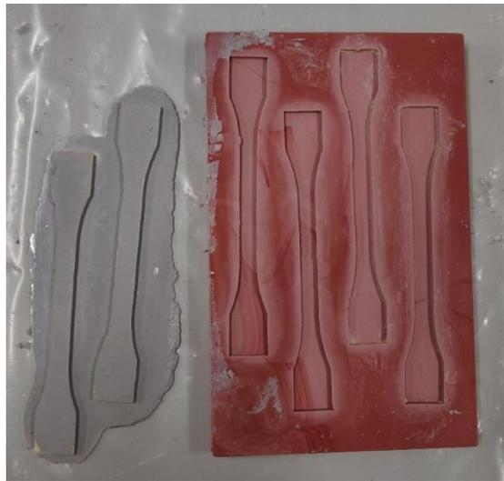
Figure 8: Molding process of Sikadur30® adhesive in silicone molds
