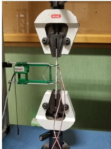
Figure 2: Traction test with specimen of adhesive Sikadur30
