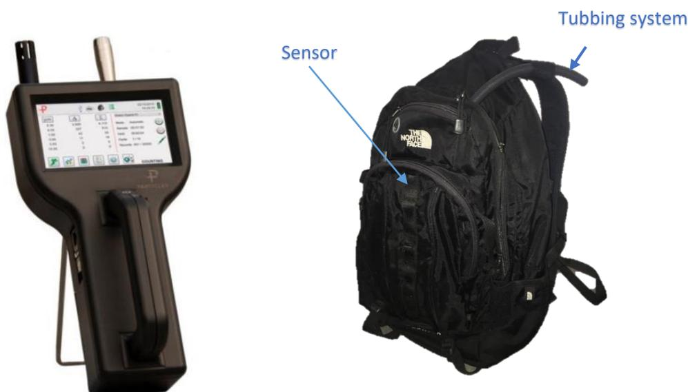
Figure 10 Graywolf Particle Counter 3500 and adapted backpack with the sensor. Source: left picture from Graywofl website. Right picture from own elaboration.
