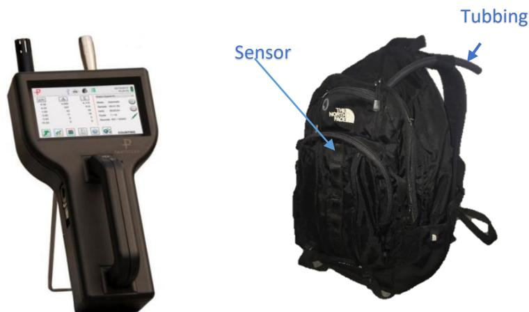
*Graywolf Particle Counter 3500 and adapted backpack with the sensor. Source: left picture from Graywofl website. Right picture from own elaboration.*
