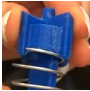
Figure 61. Spring catching the ridge of the cam pin
