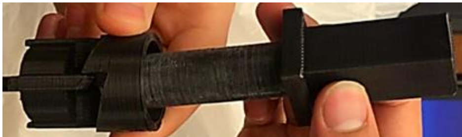
Figure 63. Second design of cam mechanism, 3D printed
