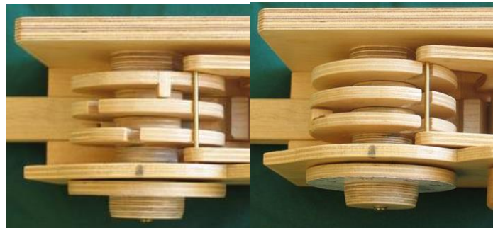
Figure 11. Inside mechanism of a single-dial lock [Source: Matthias Wandel (20 th April 2008), Wooden combination lock (video file)]
