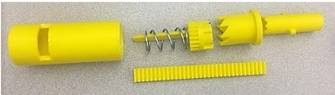
Figure 94. Cam mechanism 3D printed
