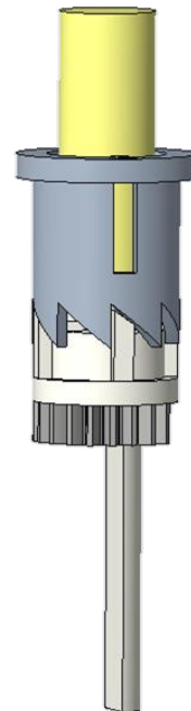
Figure 79. Cam mechanism assembled
