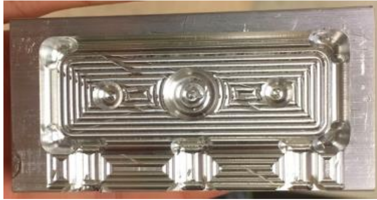
Figure 15. Picture of milled part
