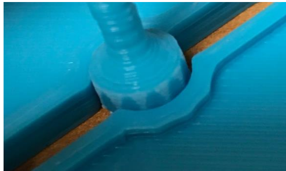
Figure 38. Sanded key inserted in the outer hole
