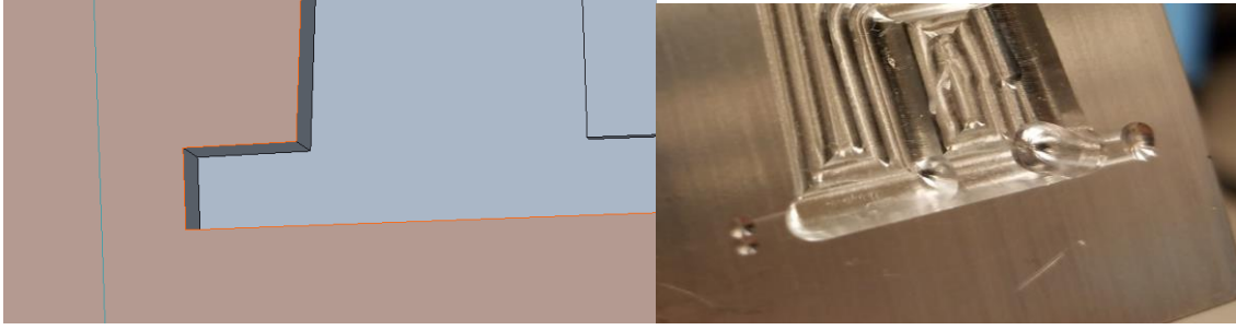
Figure 6 Creo designed base vs. Base of the machined block
