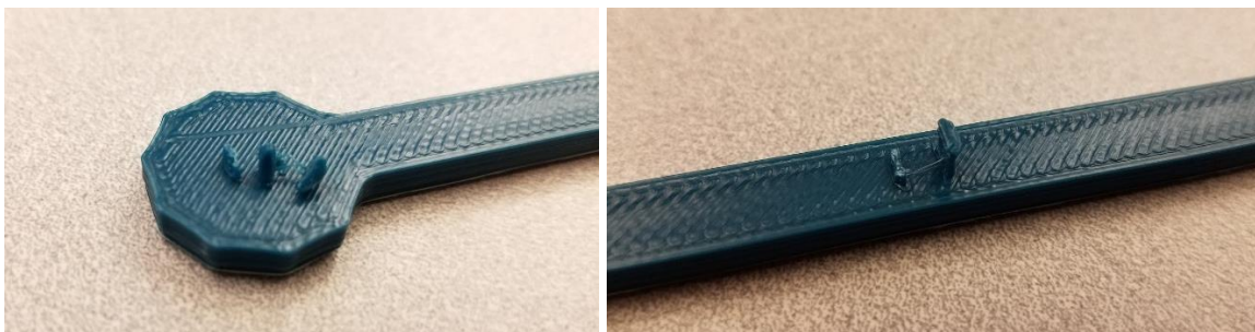
Figure 30 Failure of the first snap-fit design
