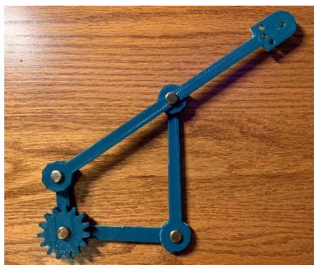
Figure- 4 Last four-bar system iteration
