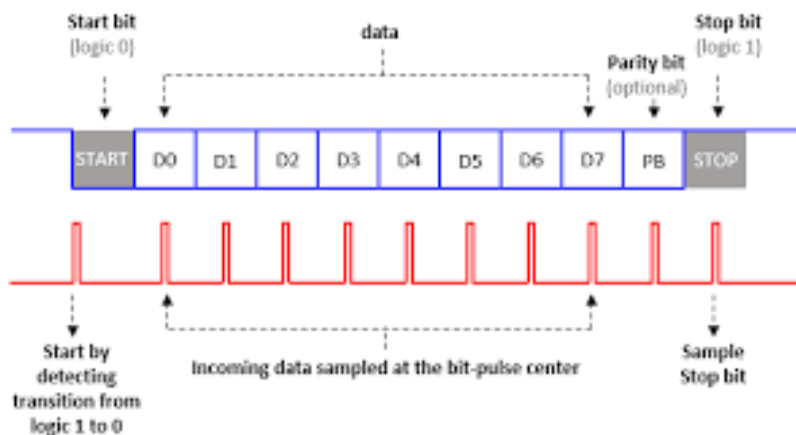
Fig. 26 UART protocol (solitontech.com)
