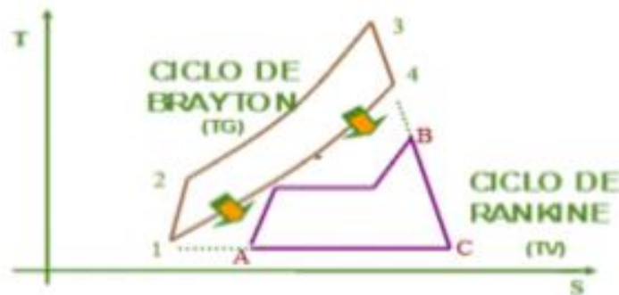
Figure 4, Brayton and Rankine Cycle, Source [ http://27.wire.karneval-lastrup.de/diagram-of-the-gas-cycle.html ]
