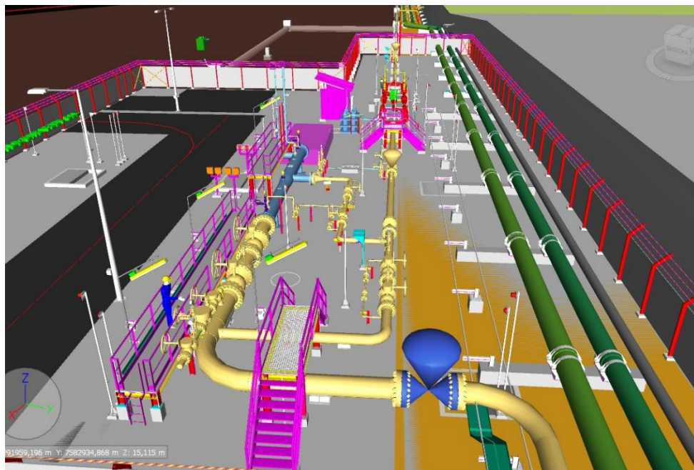
Figure 32- Side view of the Metering Station, Source [Internal design]
