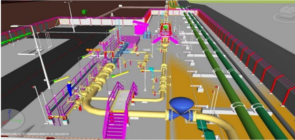
Figure 5- Natural Gas Metering Station, Source [Internal design]
