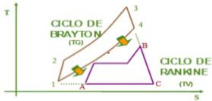
Figura 1, Ciclo de Brayton y Rankine, Fuente [ http://27.wire.karneval-lastrup.de/diagram-of-the-gas-cycle.html ]
