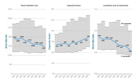
Figure 1.3: Onshore wind global weighted average total installed costs, capacity factors and LCOE, 2010–2018. Source [5].
