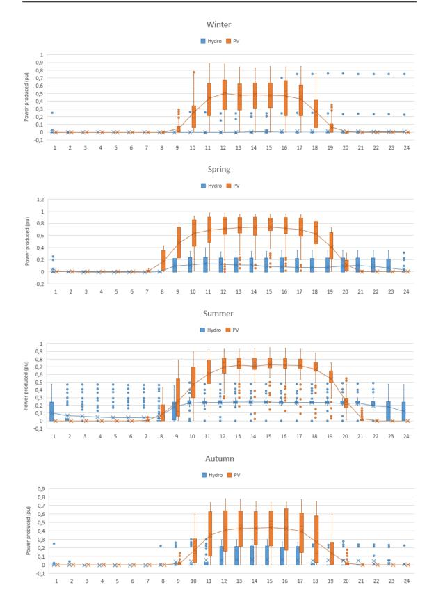
Figure B.2: Dispersion of hydro and PV production in each season and during each hour of the day for the HYDRO II power plant.
