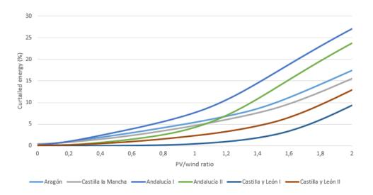
Figure A.11: Percentage of curtailed energy depending on the ratio PV/wind for all the wind power plants.
