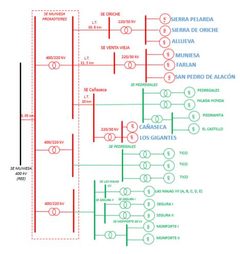
Figure 1.7: Single-line diagram of Muniesa's 400 kV substation. Source Enel Green Power (EGP) internal data.
