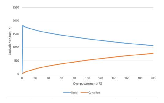
Figure A.15: Extra wind capacity equivalent hours of energy used and curtailed depending on the percentage of overpowerment for the wind power plant located in Andalucía II.
