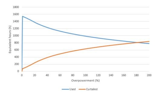
Figure A.17: Extra wind capacity equivalent hours of energy used and curtailed depending on the percentage of overpowerment for the wind power plant located in Castilla y León II.
