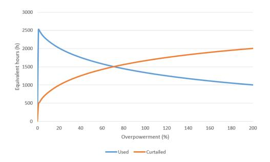
Figure 2.12: Extra wind capacity equivalent hours of energy used and curtailed depending on the percentage of overpowerment.
