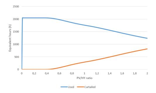
Figure 3.3: PV equivalent hours of energy used and curtailed depending on the ratio PV/HY.
