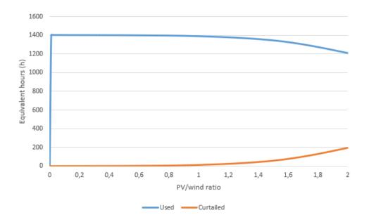
Figure A.9: PV equivalent hours of energy used and curtailed depending on the ratio PV/wind for the wind power plant located in Castilla y León I.
