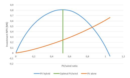
Figure 2.10: Comparison of hybrid PV and alone PV power plant net present value.
