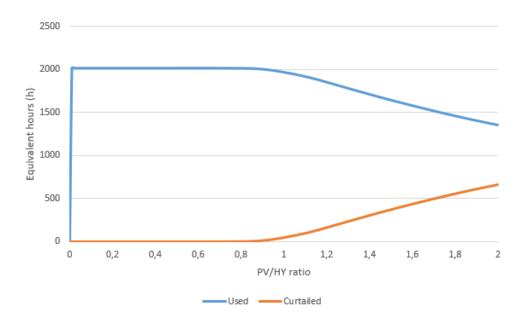
Figure B.6: PV equivalent hours of energy used and curtailed depending on the ratio PV/HY for the HYDRO II power plant.
