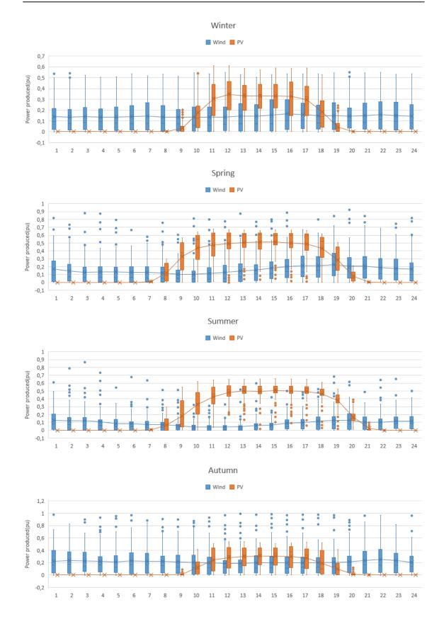
Figure A.4: Dispersion of wind and PV production in each season and during each hour of the day for the wind power plant located in Castilla y León I.
