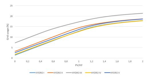
Figure B.10: Percentage of grid usage depending on the ratio PV/HY for all the hydro power plants.
