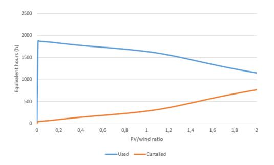
Figure A.7: PV equivalent hours of energy used and curtailed depending on the ratio PV/wind for the wind power plant located in Andalucía I.
