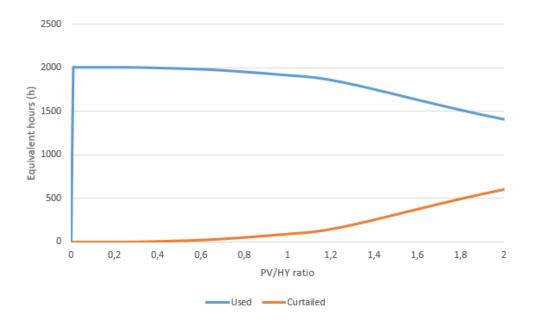
Figure B.7: PV equivalent hours of energy used and curtailed depending on the ratio PV/HY for the HYDRO IV power plant.
