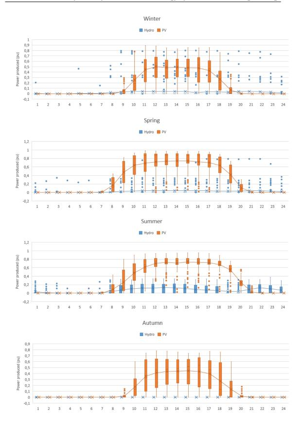
Figure B.1: Dispersion of hydro and PV production in each season and during each hour of the day for the HYDRO I power plant.
