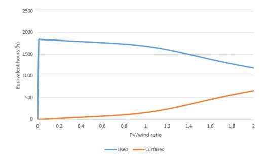
Figure A.8: PV equivalent hours of energy used and curtailed depending on the ratio PV/wind for the wind power plant located in Andalucía II.
