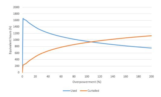
Figure A.14: Extra wind capacity equivalent hours of energy used and curtailed depending on the percentage of overpowerment for the wind power plant located in Andalucía I.
