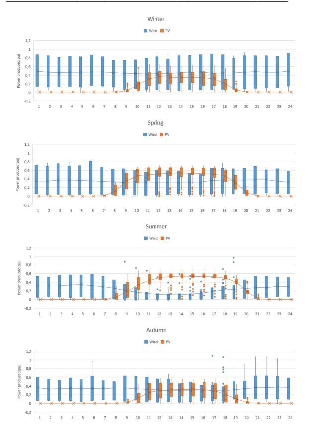
Figure A.1: Dispersion of wind and PV production in each season and during each hour of the day for the wind power plant located in Castilla la Mancha.
