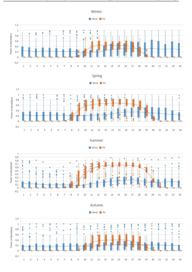
Figure A.3: Dispersion of wind and PV production in each season and during each hour of the day for the wind power plant located in Andalucía II.
