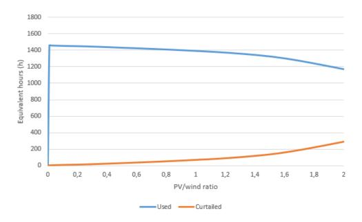
Figure A.10: PV equivalent hours of energy used and curtailed depending on the ratio PV/wind for the wind power plant located in Castilla y León II.
