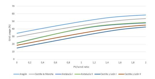
Figure A.12: Percentage of grid usage depending on the ratio PV/wind for all the wind power plants.
