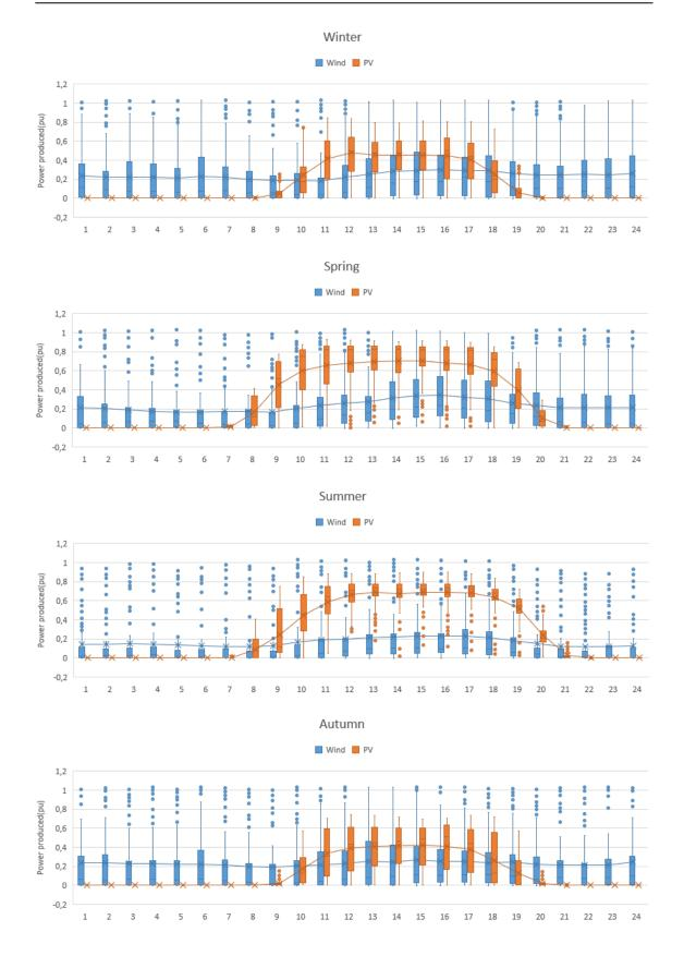
Figure A.2: Dispersion of wind and PV production in each season and during each hour of the day for wind the power plant located in Andalucía I.
