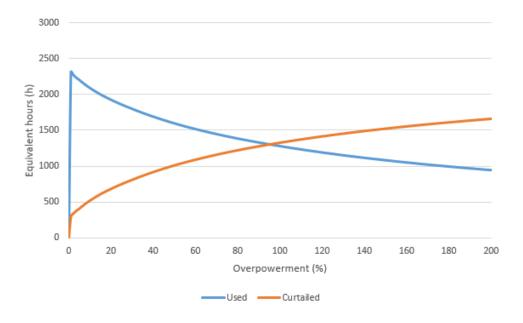
Figure A.13: Extra wind capacity equivalent hours of energy used and curtailed depending on the percentage of overpowerment for the wind power plant located in Castilla la Mancha.
