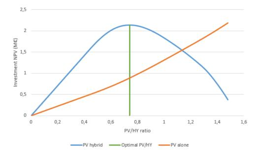
Figure 3.7: Comparison of hybrid PV and alone PV power plant net present value.
