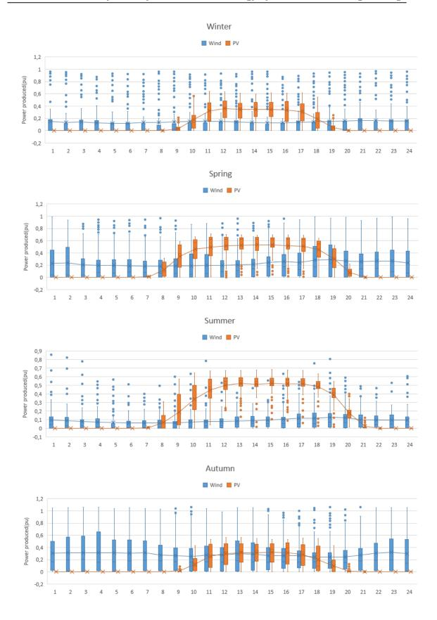
Figure A.5: Dispersion of wind and PV production in each season and during each hour of the day for the wind power plant located in Castilla y León II.
