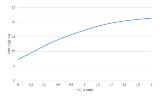
Figure 3.5: Percentage of grid usage depending on the ratio PV/HY.
