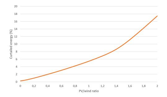
Figure 2.7: Percentage of curtailed energy depending on the ratio PV/wind.
