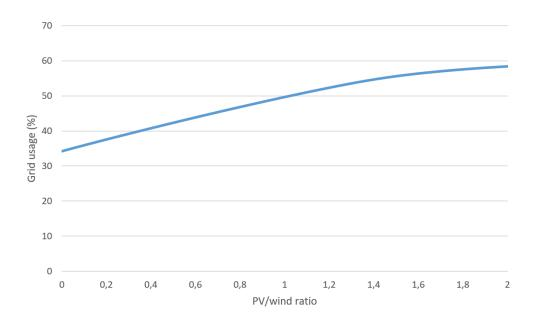
Figure 2.8: Percentage of grid usage depending on the ratio PV/wind.
