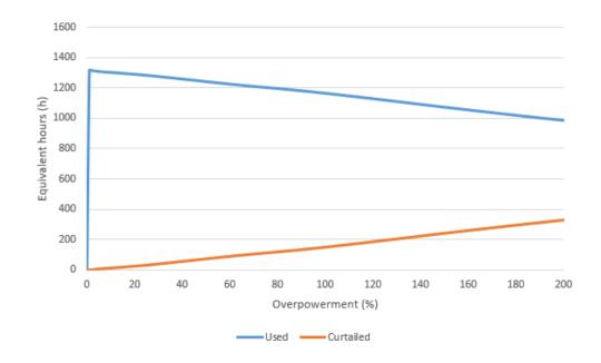
Figure A.16: Extra wind capacity equivalent hours of energy used and curtailed depending on the percentage of overpowerment for the wind power plant located in Castilla y León I.
