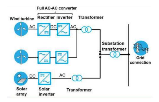
Figure 2.1: Scheme of a AC-coupled installation. Source BNEF [11].
