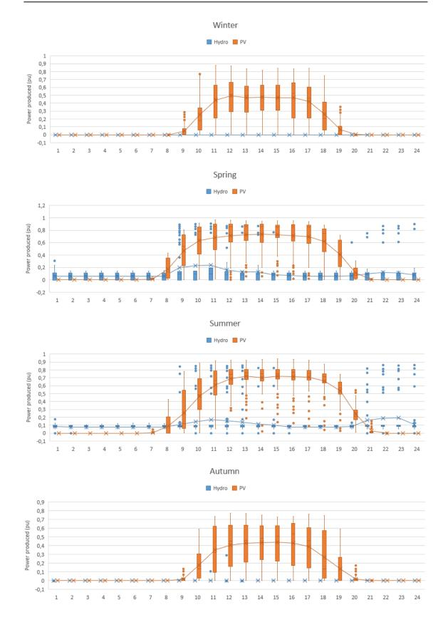
Figure B.4: Dispersion of hydro and PV production in each season and during each hour of the day for the HYDRO V power plant.
