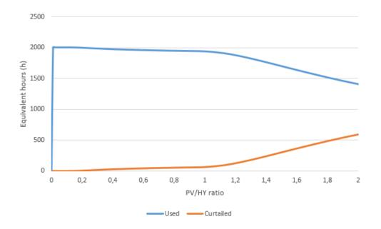
Figure B.8: PV equivalent hours of energy used and curtailed depending on the ratio PV/HY for the HYDRO V power plant.
