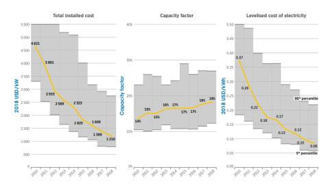
Figure 1.2: PV global weighted average total installed costs, capacity factors and LCOE, 2010–2018. Source [5].
