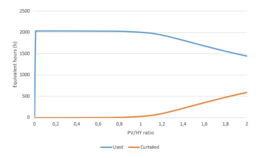
Figure B.5: PV equivalent hours of energy used and curtailed depending on the ratio PV/HY for the HYDRO I power plant.
