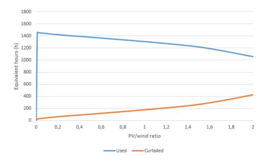
Figure A.6: PV equivalent hours of energy used and curtailed depending on the ratio PV/wind for the wind power plant located in Castilla la Mancha.
