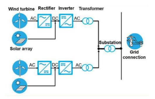
Figure 2.2: Scheme of a DC-coupled installation. Source BNEF [11].
