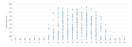
Figure 2.11: Dispersion of the excess energy in each hour of the year.
