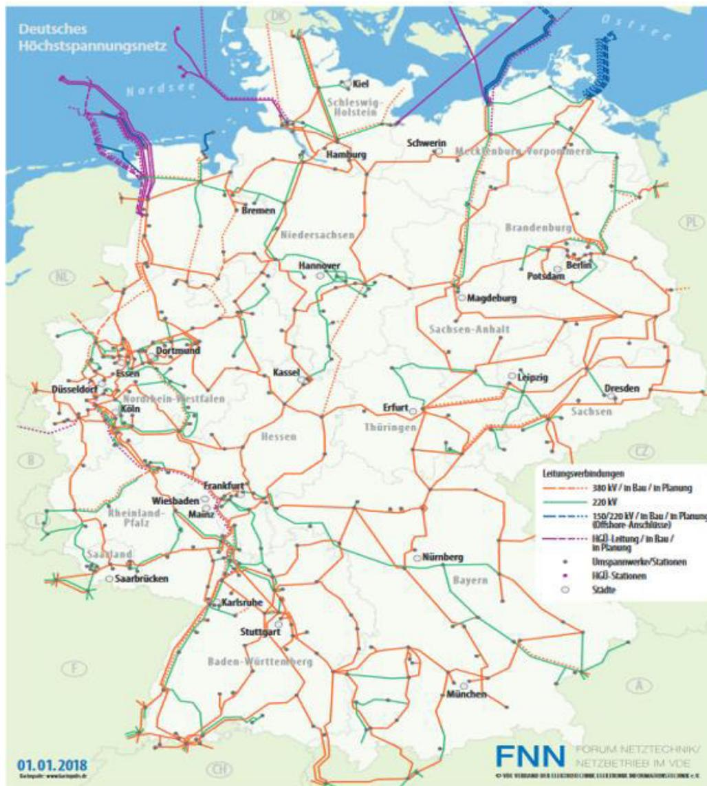
Figure 5.22: Electrical grid in Germany [66]
