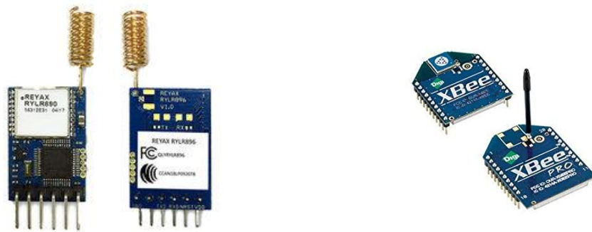
Figure (56). Picture of both the Lora Module (Left) and XBee Module (Right).
