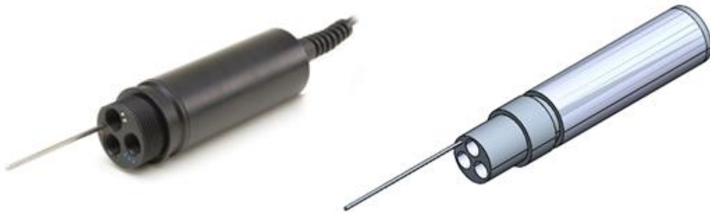
Figure (33). Thermocouple sensor vs. its CAD model.
