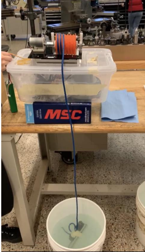
Figure (53). First Test for the Iteration 1 Sensor Deployment Mechanism.
