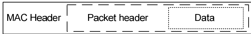
Figure 7.8: Generic scheme of the a MAC frame. Dashed lines stand for optional parts.
