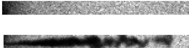
*Figure 17. Comparison of the 150x11 pixels region for a frame without a spray (top) and a frame with a spray (bottom)*
