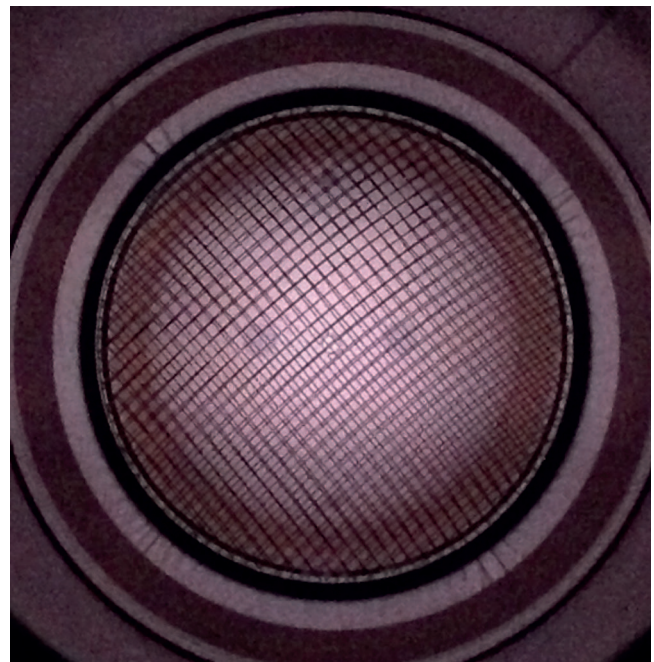
FIG. 12. Digital photograph of the plasma sustained in the optimized design plasma chamber without magnetic field.
