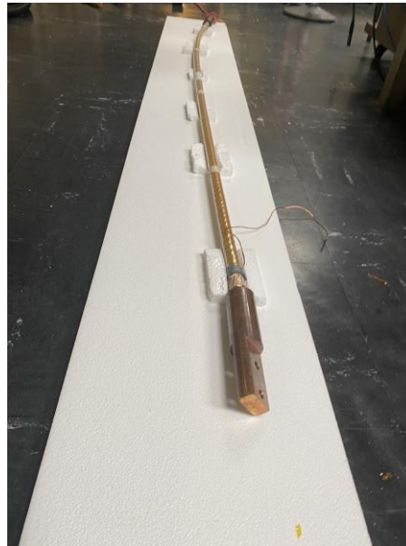
Figure 7. 21: Cable core resting on spacers
