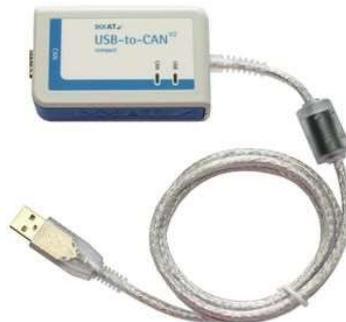
Figura 47: USB-to-CAN V2 compact de IXAAT. [43]
