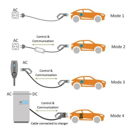
Figure 15. Four charging modes for EV. Source: [29]
