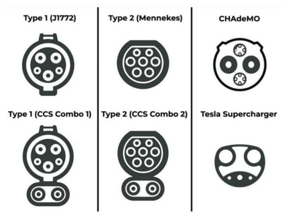
Figure 14. Main types of EV chargers. Source: [28]
