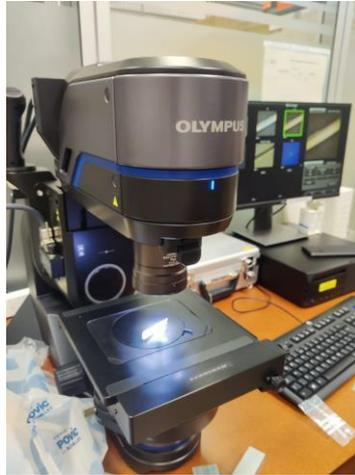
*Figura 44. Microscopio digital Olympus DSX1000.*
