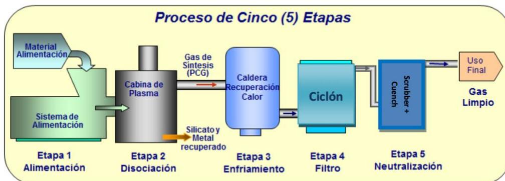
This system has been designed in the most efficient way possible, including a system to take advantage of heat losses through a Rankine cycle. After each of these stages, a synthetic gas with a high concentration of hydrogen -around 50%- is obtained, which is suitable for use as fuel. For the design of this project in the chosen city, a constant flow of about 35,000 kg of this gas per hour has been estimated, which corresponds to about 3,000 kg of hydrogen.
