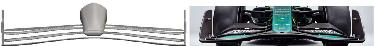
*Figure 42: AMR22 Frontwing CAD vs Real*
