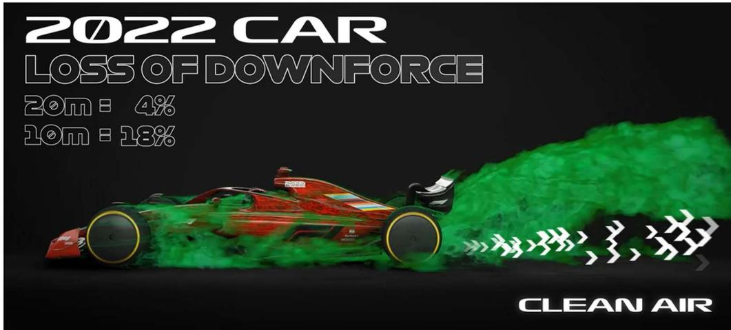
*Figure 4: Loss of downforce following a 2022 F1 car*
