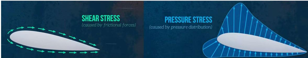
*Figure 34: Shear and Pressure stresses*
