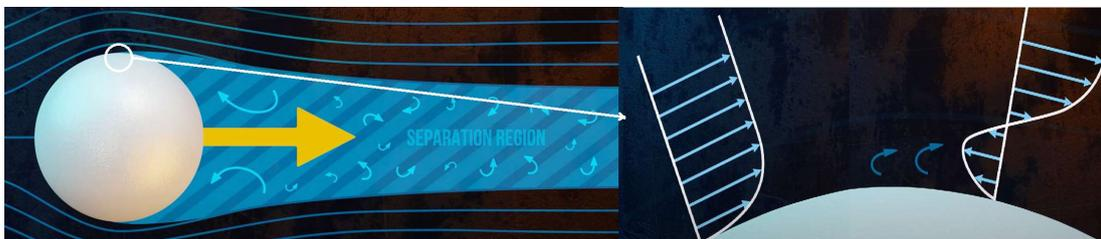
*Figure 35: Flow separation*
