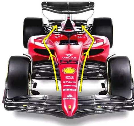
*Figure 9: F1-75 Sidepods Air Flow Streamline*
