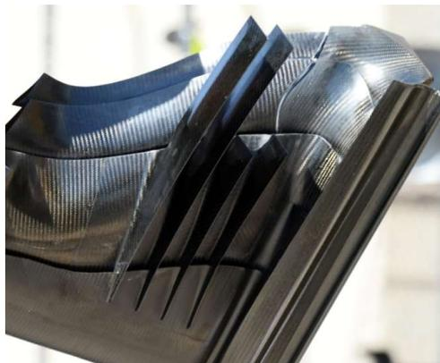
*Figure 26: Strakes in Front Wing*
