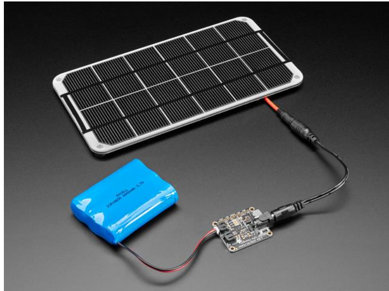
Figure 9. Solar charger connected to the battery and solar panel [11]
