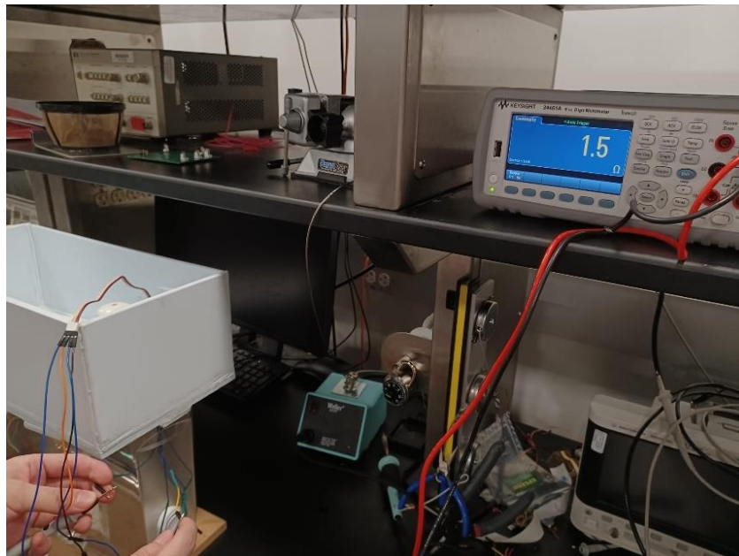
Figure 29. Short between signal and ground
