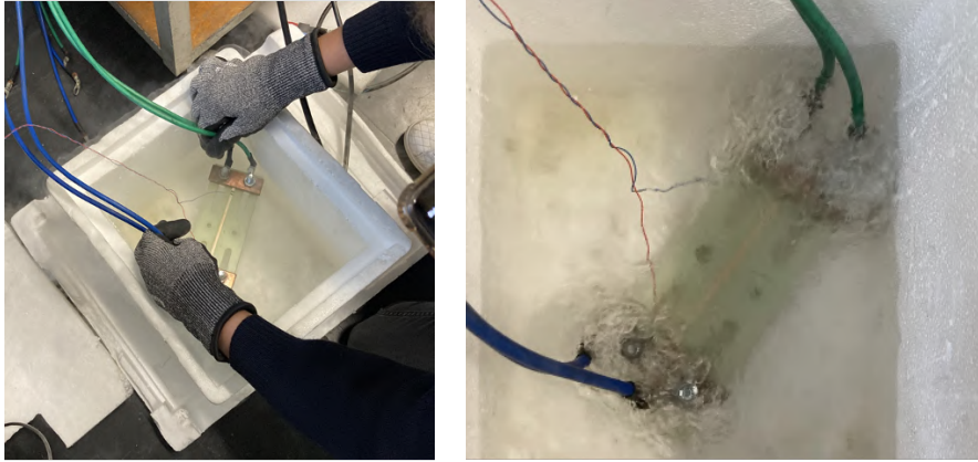
Figure 4.3: Electrical installation in liquid nitrogen
