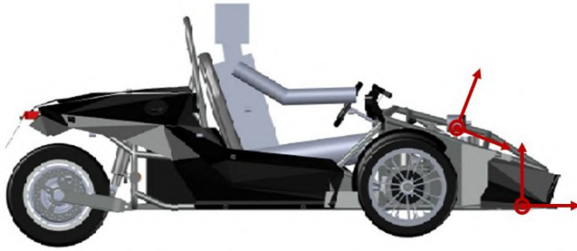
Figure 5.1 Displacement between gyroscope and accelerometer coordinate system
