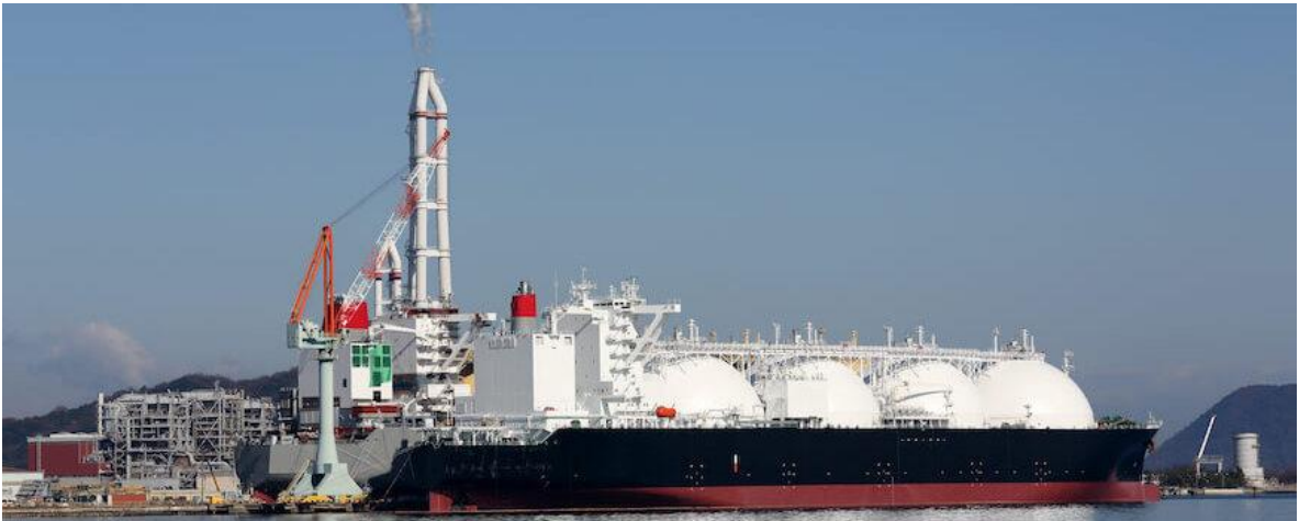
Figure 2.4. LNG tanker used for marine transport [4].
