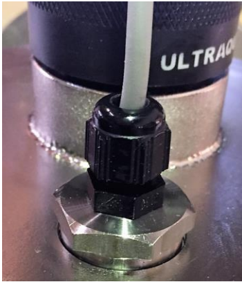
Temperature sensor, SS reactors.
