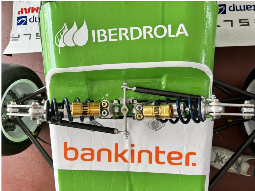
This is the Z-shaped system in the front axle, now the U-shaped system in the rear axle will be shown:
