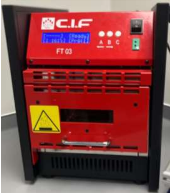
Figure 26: Furnace used to solder the components onto the PCB.
