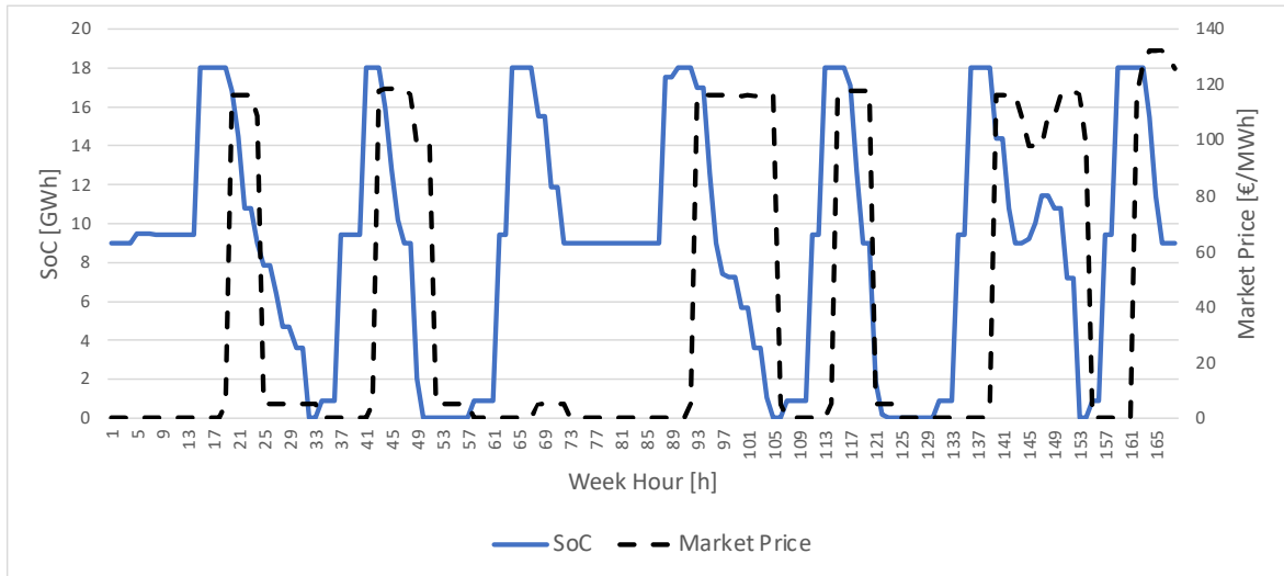
Figure 5. Correlation between the market price fluctuation and the battery's operation with five segments in the degradation cost function
