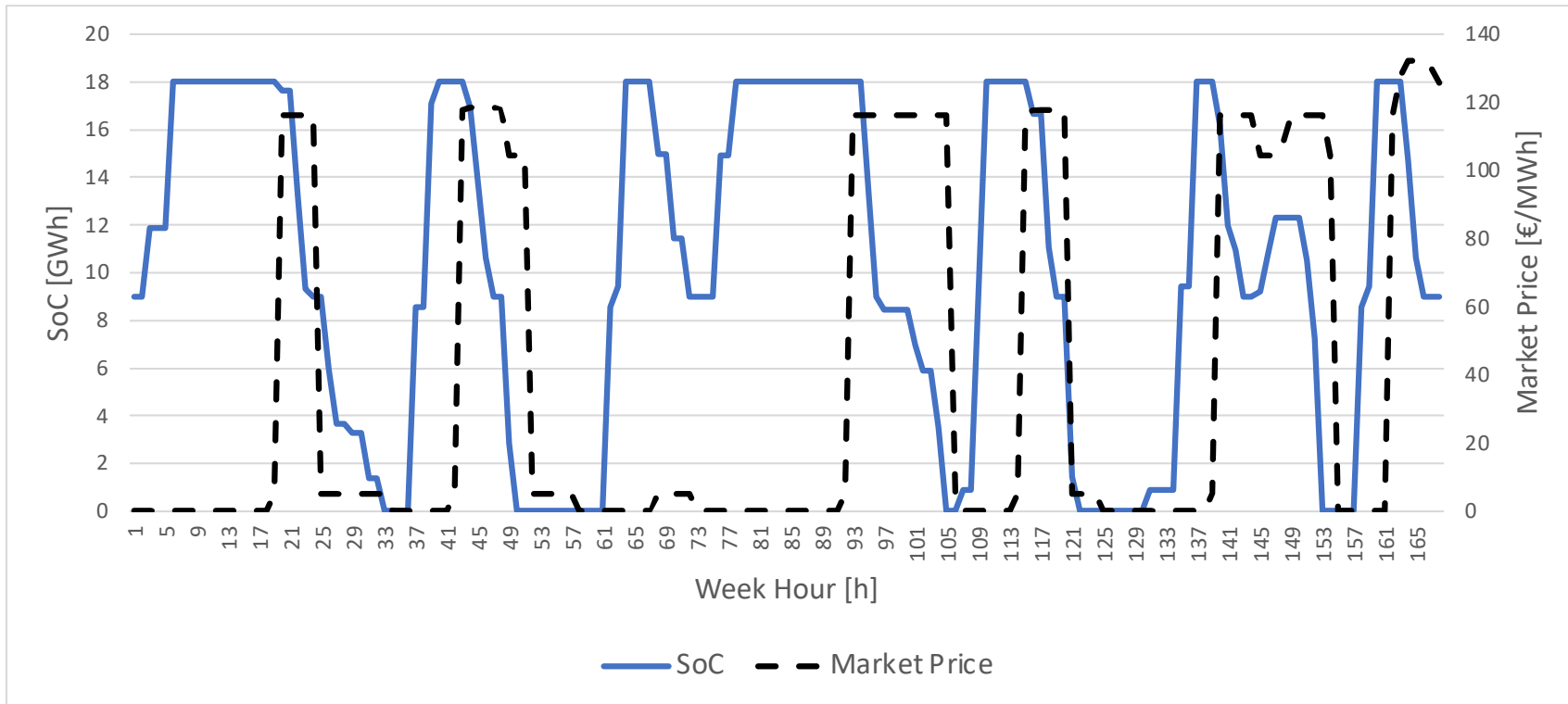
Figure 4-9. Correlation between the market price fluctuation and the state of charge of the battery when the cycle aging cost is approximated by a single segment
