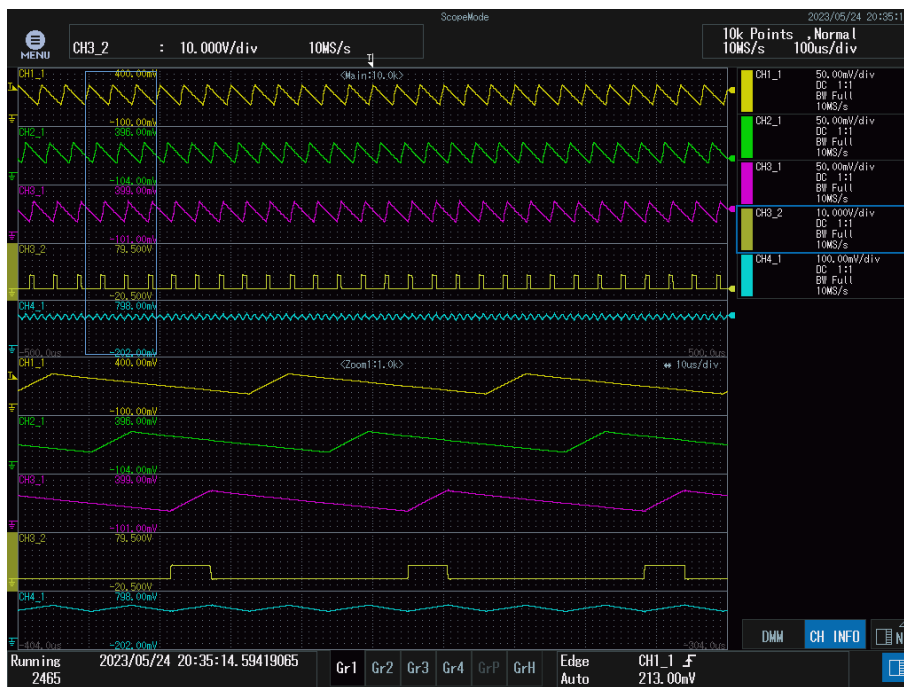
Figure 3: Open loop test waveforms open loop nominal duty point. CH1_1, CH2_1, CH3_1 correspond to the current of phase A, B and C respectively. CH4_1 represents the sum current of the three currents and CH3_2 the phase C triggerings.
