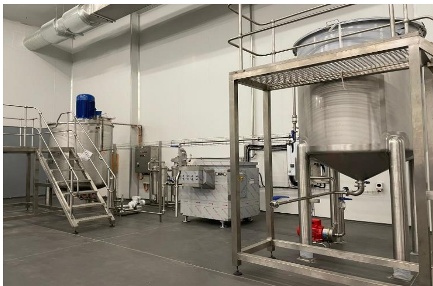
Illustration 1. Example of vessel for mixture with pumps, piping and other elements. Source: Iberchem employee
