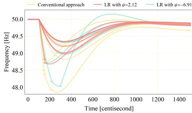
**FIGURE 11** Frequency response after outages for a random hour with UFLS
