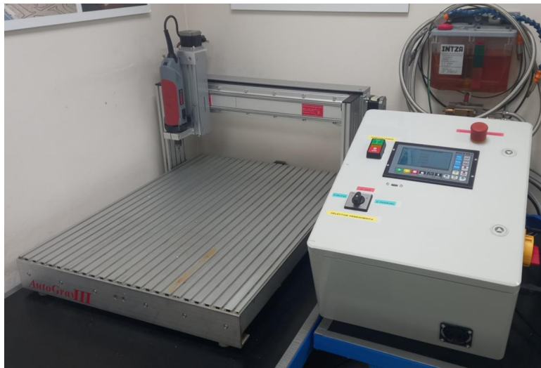
Illustration: Controller and router after finishing the project [Own work]
