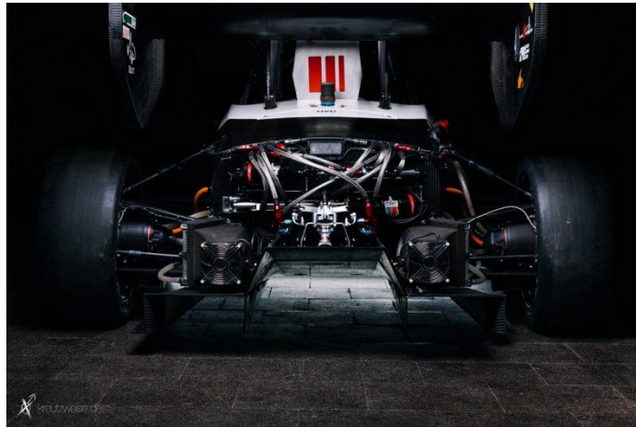
Figure 19. The fully decoupled hydraulic suspension of AMZ's Formula student prototype. [15]
