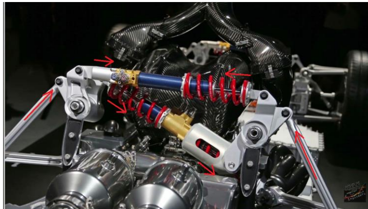
Figure 34. Diagram showing the compression of the heave spring and no reaction of the roll spring when both tyres move equally. [16]
