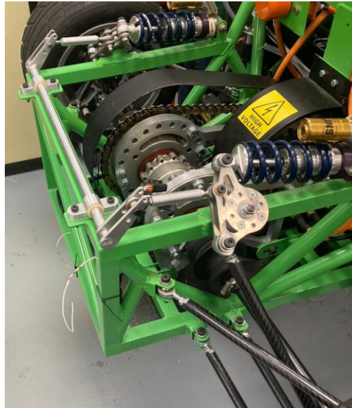
Figure 17. The rear u-shape ARB of the ISC's IFS-06
