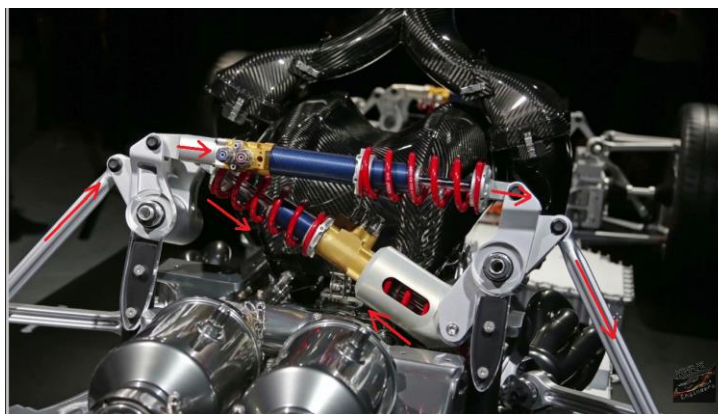
Figure 35. Diagram showing the compression of the roll spring and no reaction of the heave spring when both tyres move opposite. [16]
