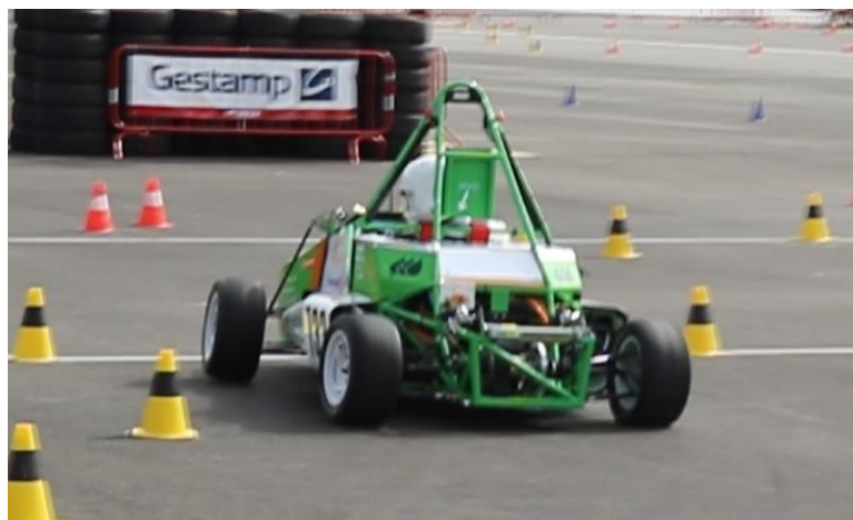
Figure 25. Image of the car oversteering at last year's Formula Student Spain Skidpad event
