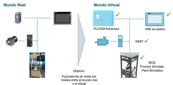
Figura 5. Software in the Loop [5]
