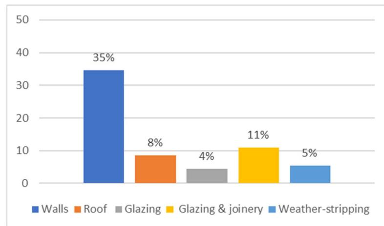
**Figure 3.** Reduction in the required heating demand [%] in Madrid according to the passive measure implemented.
