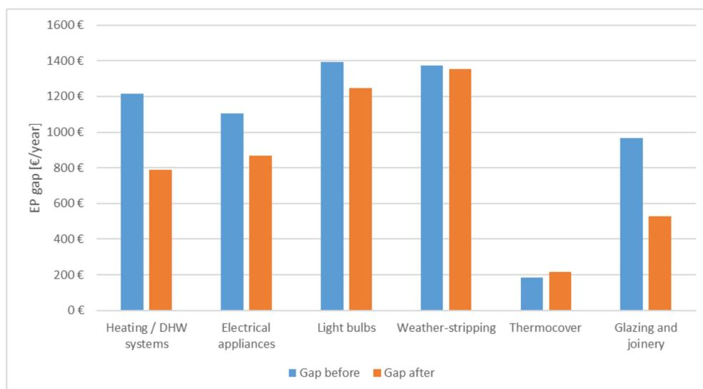
**Figure 13.** EP gap before and after retrofitting according to the implemented measure.
