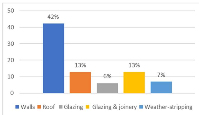
**Figure 2.** Reduction in the required heating demand [%] in La Coruña according to the passive measure implemented.
