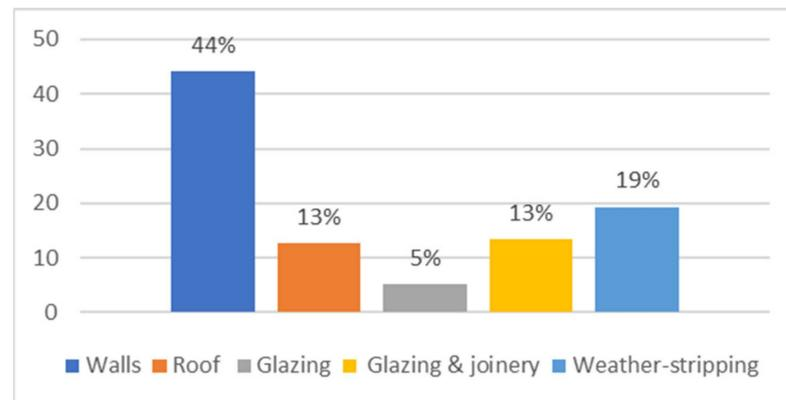
**Figure 4.** Reduction in the required heating demand [%] in Sevilla according to the passive measure implemented.
