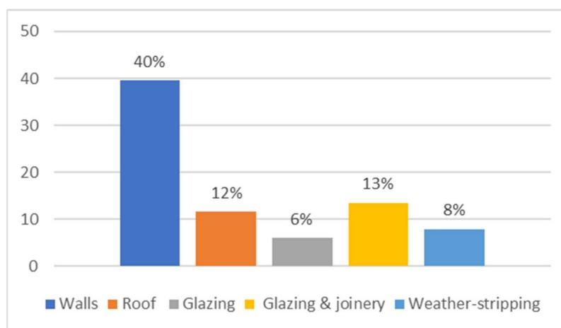
**Figure 1.** Reduction in the required heating demand [%] in Barcelona according to the passive measure implemented.
