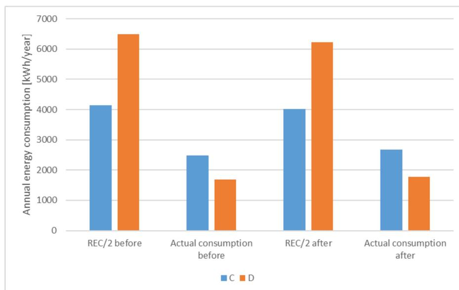
**Figure 10.** Average of half of the required energy consumption (REC/2) and actual consumption before and after retrofitting according to the winter climate zone (ZCI).
