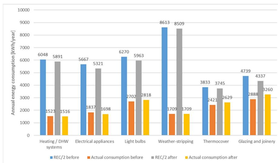
**Figure 9.** Average of half of the required energy consumption (REC/2) and actual consumption before and after retrofitting according to the type of measure implemented.
