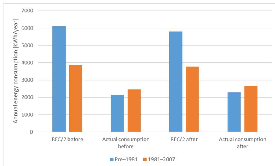
**Figure 11.** Average of half of the required energy consumption (REC/2) and actual consumption before and after retrofitting according to the building age.
