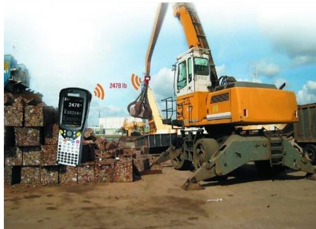
Figure 6: example of a weighing grapple operating by radio link
