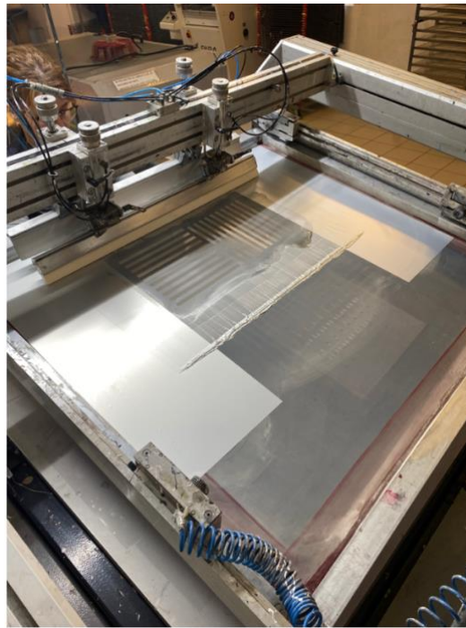
Figure 15: screen printing using silver ink
