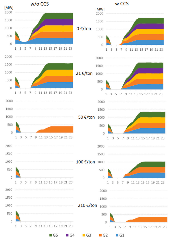
Fig. 11. Hourly scheduling with different values of T_xCO_2 = \{0, 21, 50, 100, 210\} €/ton with and without CCS.
