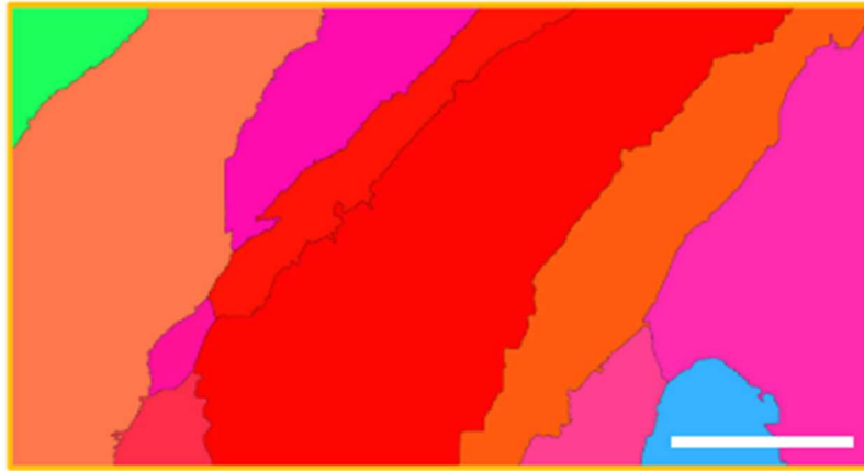
Figure 20: Morphology associated to columnar grains [38]
