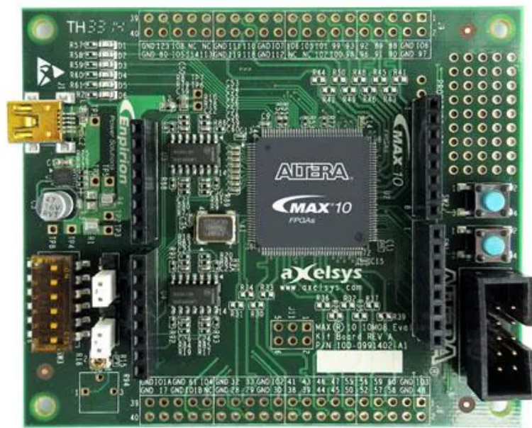
Figure 7. Intel MAX 10 - 10M08 Evaluation Kit [17].
