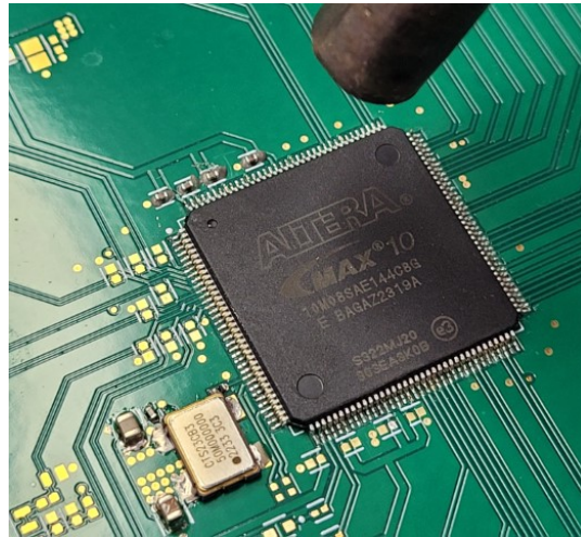
Figure 23. FPGA chip, Decoupling Capacitors, and Oscillator being soldered to the Board.
