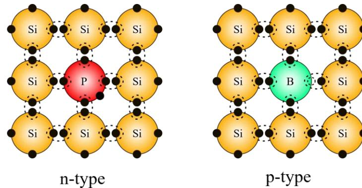
Figure 2: Molecular structure of doped silicon with phosphorous and boron [2]
