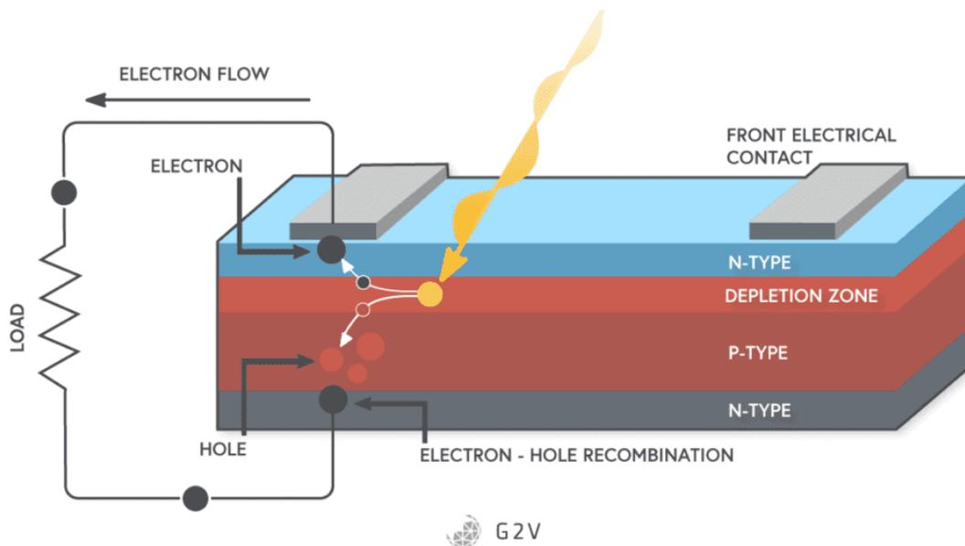
*Figure 1: Schematic diagram of a solar cell [1]*
