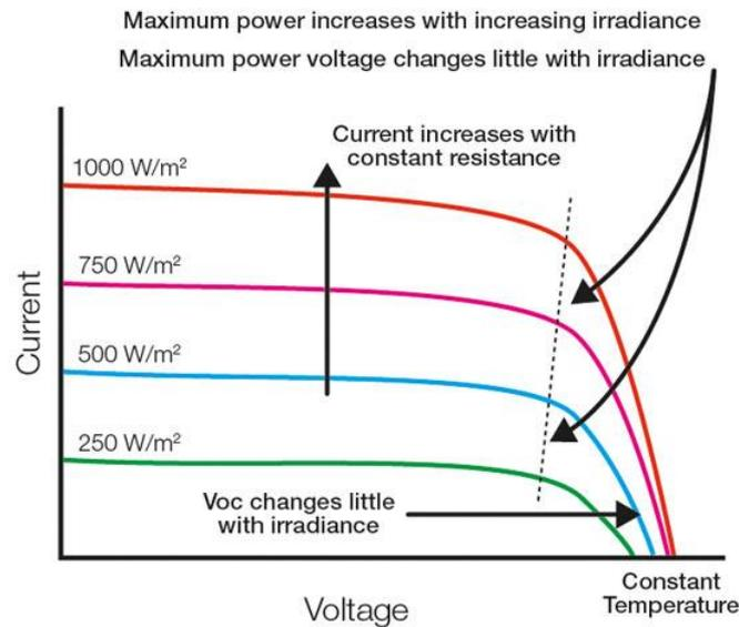
Figure 9: *I-V* curves with varying irradiance and constant temperature [8]
