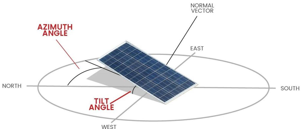
*Figure 19: Tilt and azimuth angles in a solar panel [19]*
