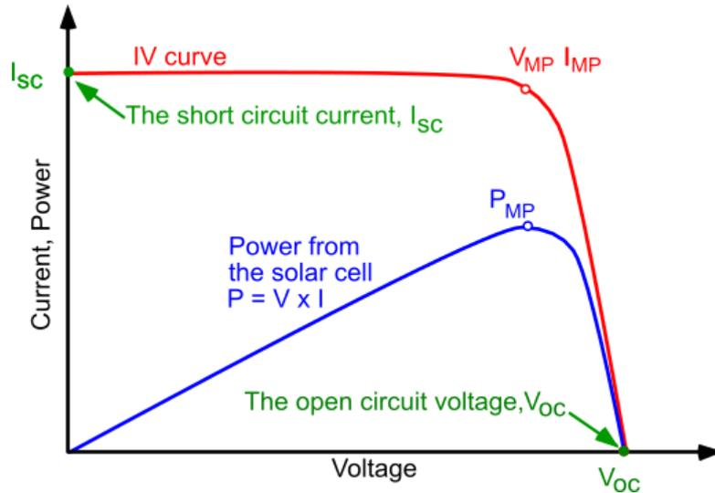
Figure 6: Current-voltage ( $I$ - $V$ ) curve of a solar cell [7]
