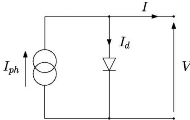
Figure 5: Ideal PV cell equivalent circuit [6]
