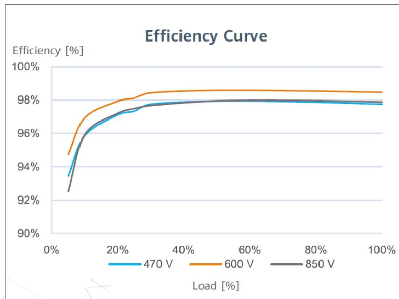
Figure 15: Efficiency curves of a Huawei SUN2000 inverter [9]
