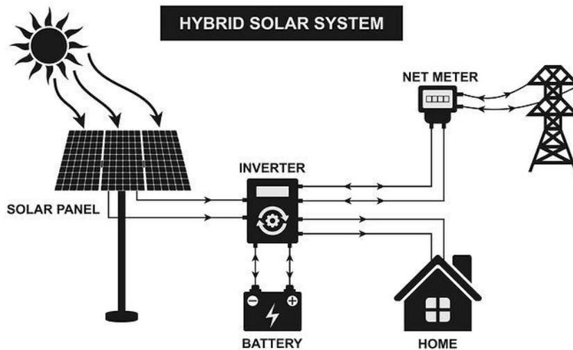
Figure 14: Schematic of a hybrid inverter topology [14]
