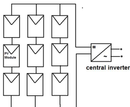
Figure 11: Schematic of a central inverter topology [10]
