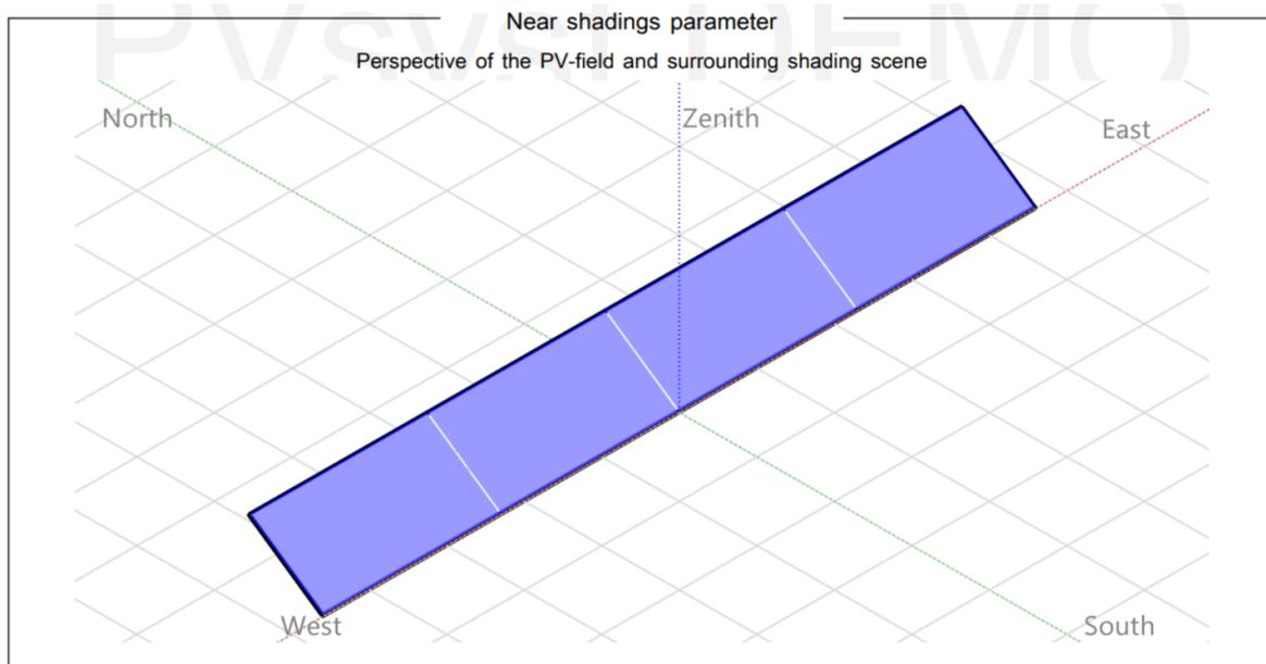
Figure 42: Fixed-tilt 35° South structure for a 2.2 kWp installation
