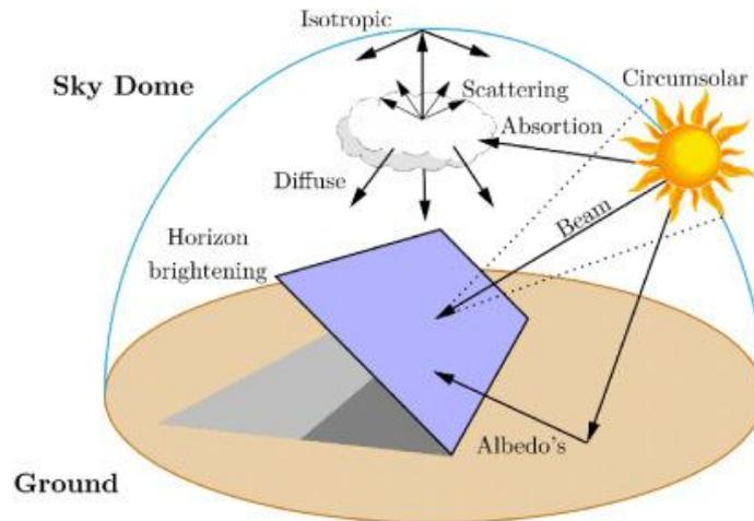
*Figure 17: Components of solar irradiance on a tilted surface [17]*
