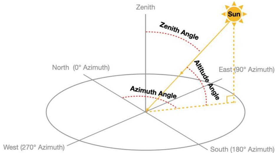
Figure 16: Schematic depicting the altitude, zenith and azimuth angles [16]
