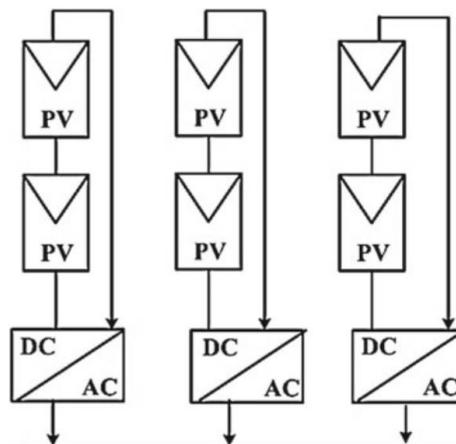
*Figure 12: Schematic of a string inverter topology [11]*
