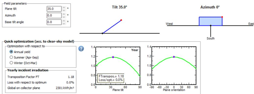
Figure 41: Optimal tilt and azimuth angles for a fixed-tilt structure according to PVsyst
