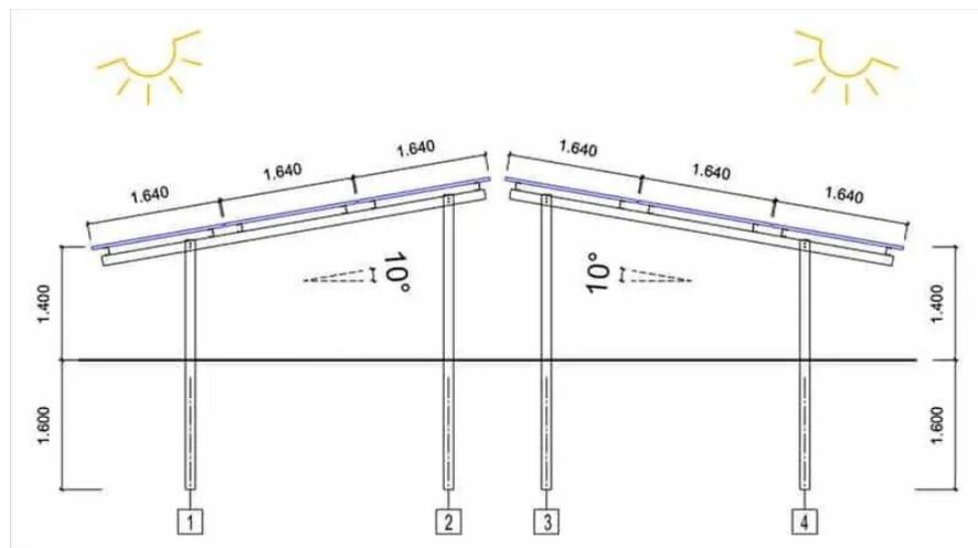
*Figure 23: East-West structure system with 10° tilt [26]*
