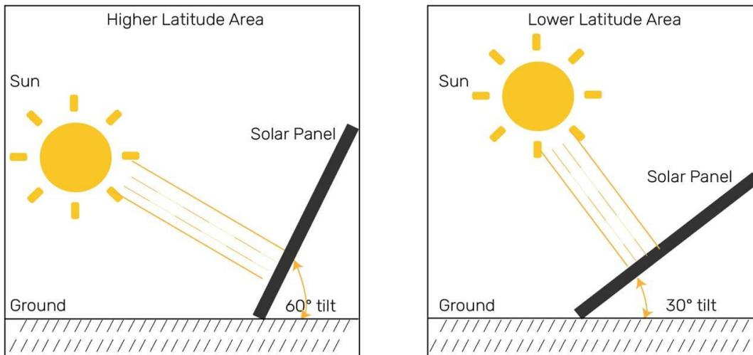
Figure 21: Tilt angles of solar panels depending on latitude [23]
