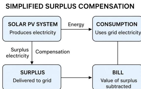
*Figure 27: Flowchart of surplus energy compensation in residential solar installations*
