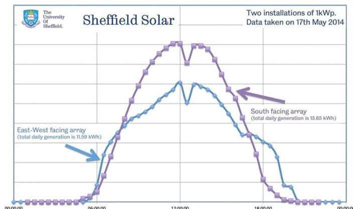
*Figure 24: Comparison between East-West oriented and South oriented PV systems [27]*
