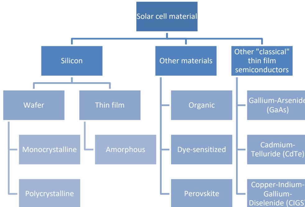
*Figure 4: Overview on different solar cell technologies*
