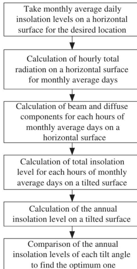
*Figure 22: Flowchart of the annual optimum tilt angle calculation algorithm [25]*
