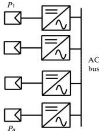
Figure 13: Schematic of a microinverter topology [11]
