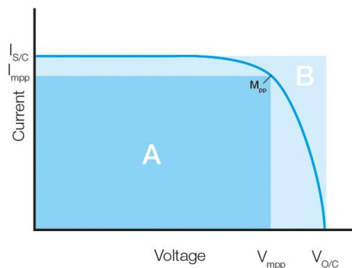
Figure 7: Representation of areas used in calculation of FF [8]
