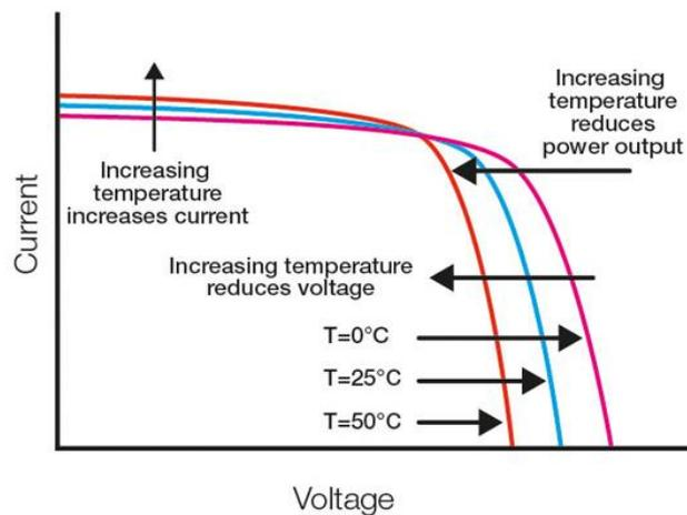
*Figure 8: I-V curves with varying temperature and constant irradiance [8]*
