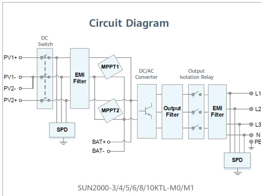
Figure 10: Circuit diagram of a Huawei SUN2000 inverter [9]
