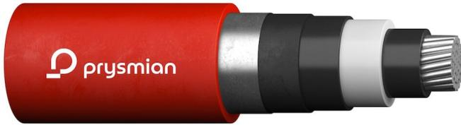
Medium voltage cables for rated voltages from 6 kV ( $U_m = 7,2$  kV) up to 30 kV ( $U_m = 36$  kV) used for industrial installations or for a distribution network. Designed for fixed installations indoors, outdoors or in buried installations. Conductor shape round, class 2 = stranded; red outer sheath
