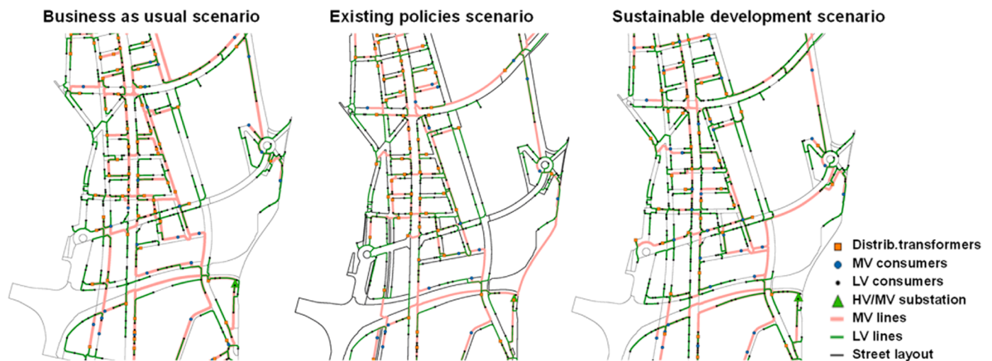
Fig. 5. Zoom of the graphical layout of the electricity distribution networks in, from left to right, the business as usual , existing policies , and sustainable development scenarios.
