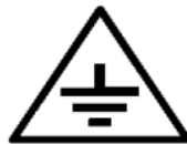
Figure 4. Grounding symbol next to the terminal.
