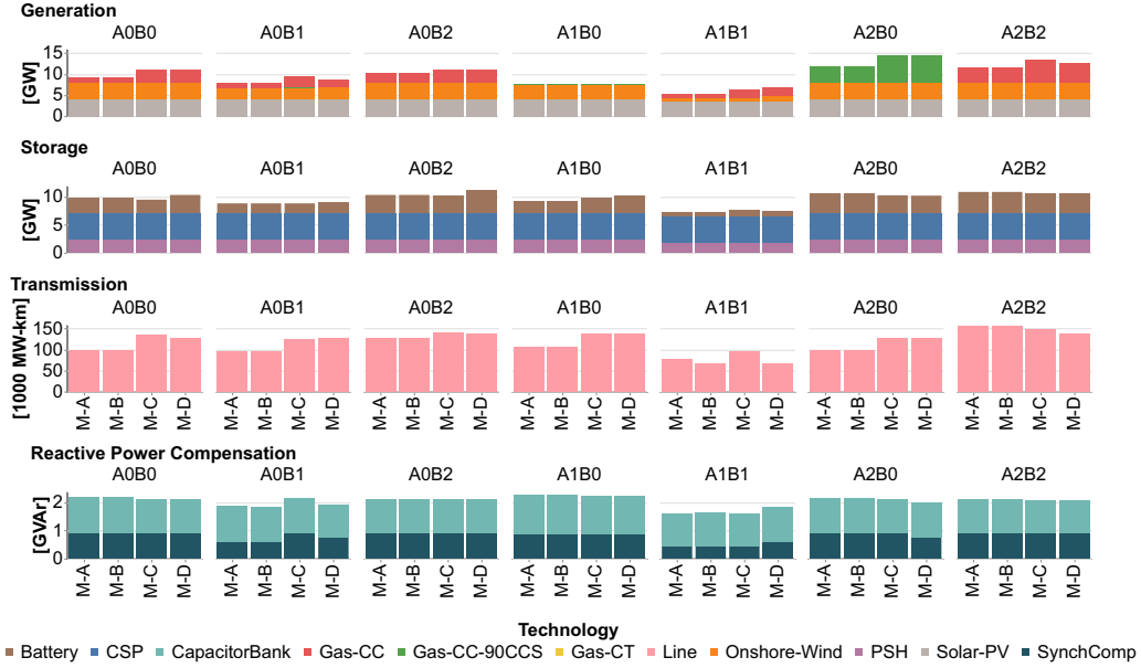
Figure 5: Installed capacity in power generation, energy storage, transmission network and reactive power compensation assets per scenario and formulation.
