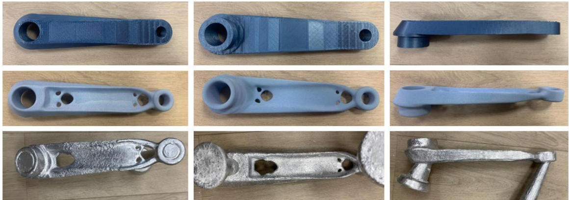
Ilustración 2: Comparison between original, optimized and cast crank arm. Own source.
