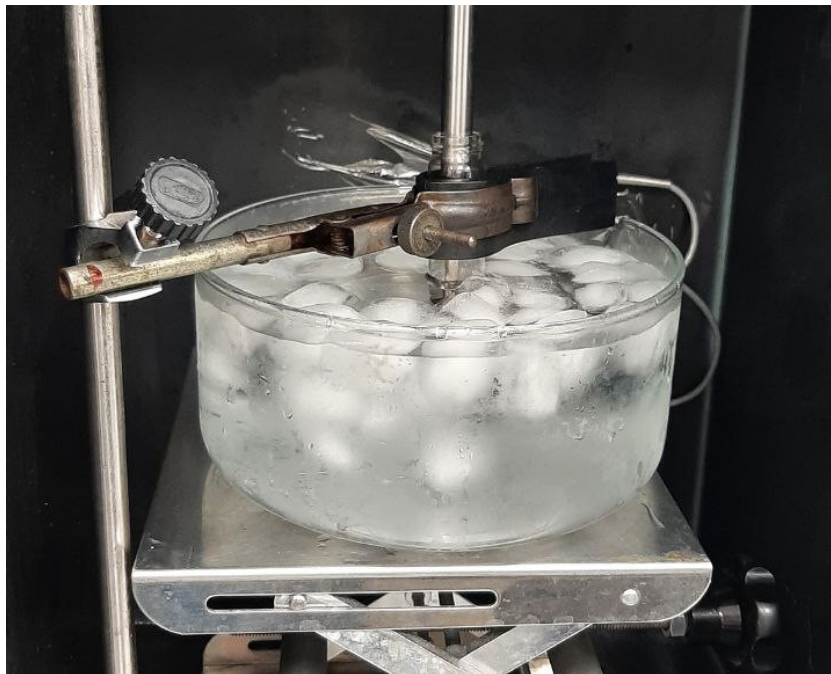
Figure 2.6. Test tube containing paraffin and nanoparticles submerged in an ice bath with the sonicator probe, ready to start the sonication process.
