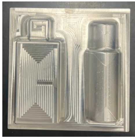
Image 5: Male mold in aluminum (Own work)
