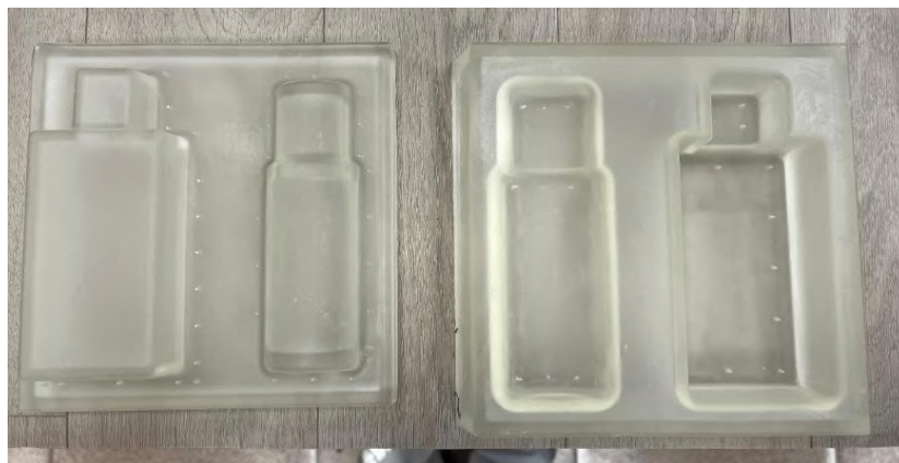
Image 6: SLA-printed molds: male (left) and female (right) (Own work)
