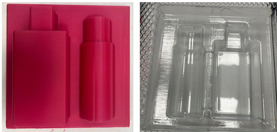
Image 7: Mold manufactured by FDM (left) and thermoformed blister obtained from it (right) (Own work)
