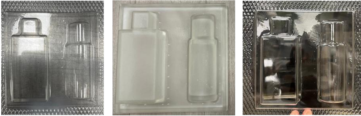
Image 8: Mold manufactured using SLA (center) and thermoformed blisters obtained from it (sides) (Own work)
