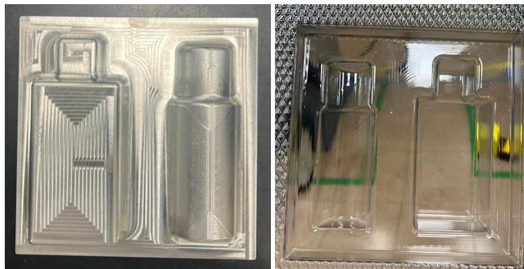
Image 10: Mold manufactured by MCNC (left) and thermoformed blister obtained from it (right) (Own work)
