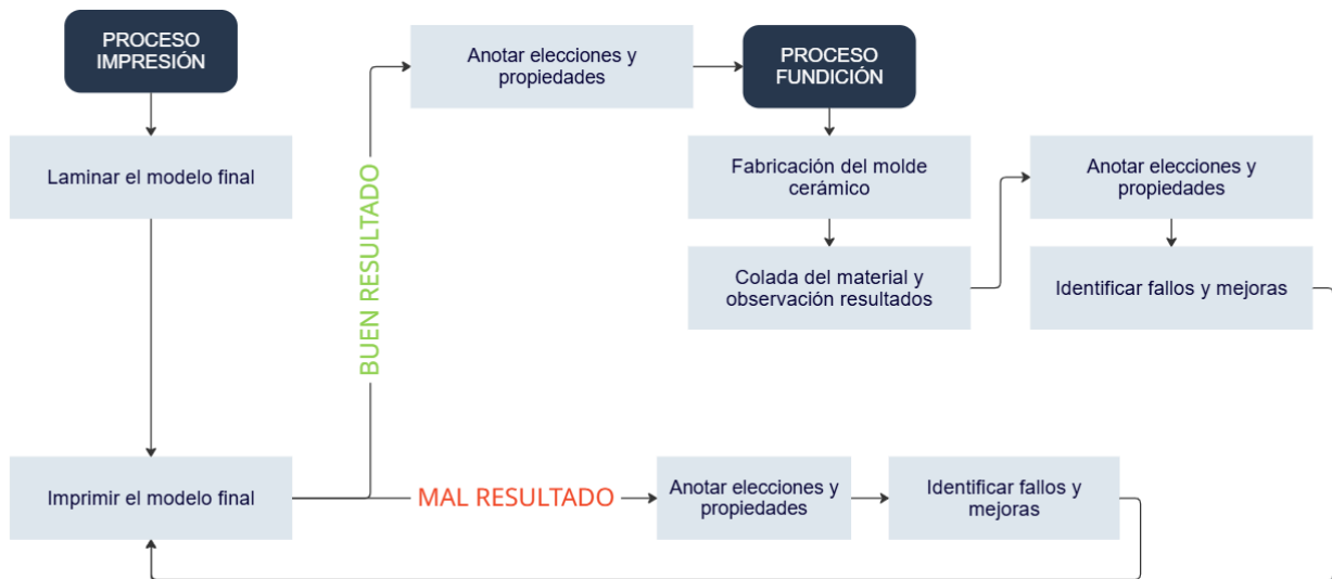
Ilustración 6: Workflow of the 3D printing and casting environment in the project (Source: Own elaboration)
